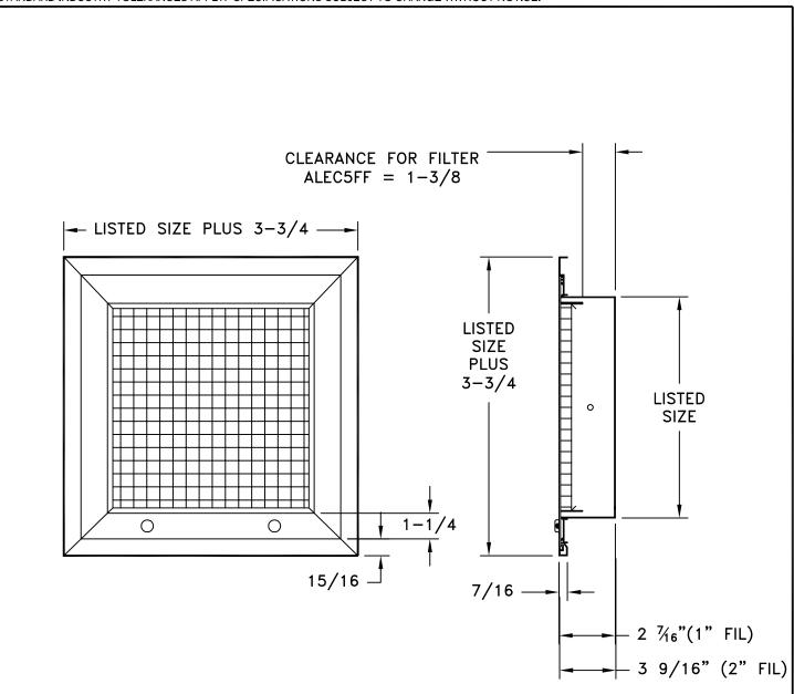
The Model ALEC5FF is a return air filter grille that has an aluminum square pattern grid providing maximum free area. ALEC5FF has a 1/2" x 1/2" x 1/2" core grid.
