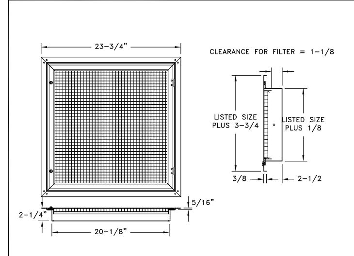
The Model ALEC5FF LAY-IN is a return air filter grille that has an aluminum1/2" x 1/2" x 1/2" square pattern grid providing maximum free area.
