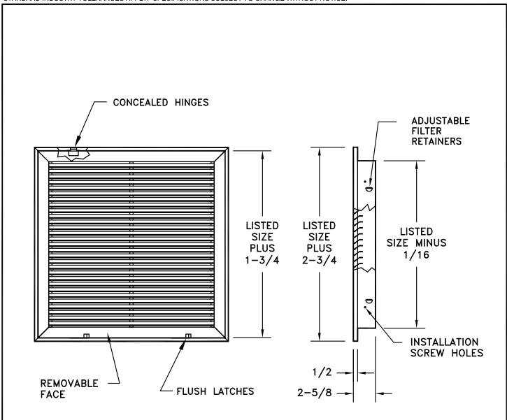
Model S90HFF or S90VFF Grille with filter frame is designed for use in all types of air conditioning systems. In addition to holding the filter, unit can be used as an access opening into small air handling units. Standard hinge location is at top of face. Standard latch is located on side opposite hinge. Standard filter frame holds 1" disposable filter (provided by others). 2" filter size also available. Steel construction. Standard finish is white.
