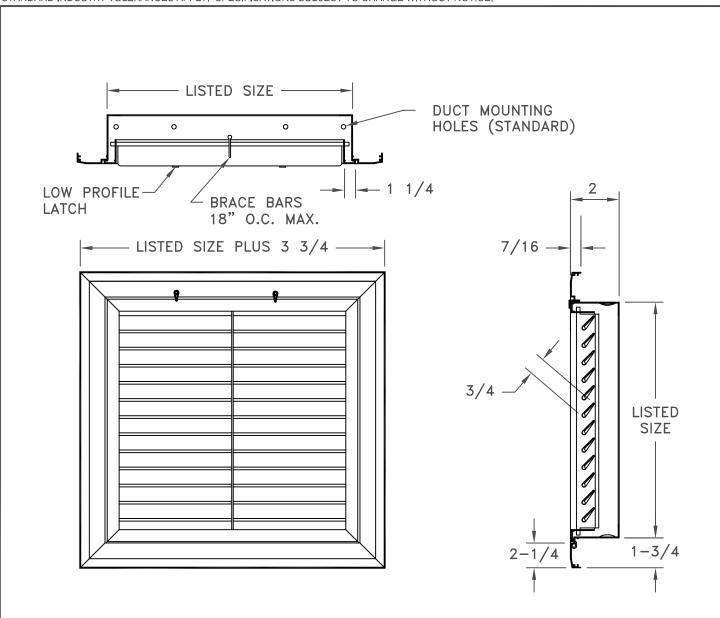
Model ALH45FF is a filter frame with fixed horizontal face bars set at 45° made of extruded aluminum construction. Optional 2-inch filter frames available. White (WHT) or clear anodized (CLR) finishes are available.
