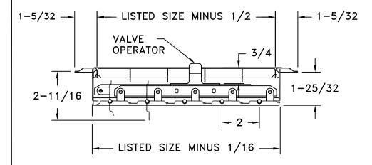
Model 830 is a heavy duty floor register. Constructed of steel, it features a smooth surface face and a toe operated multi-louvered damper. Standard finish is brown.
