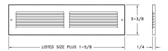
Model 827 is a stamped straight blade toe space register with mounting holes. May be used as an inlet or outlet. Standard finish is white.
