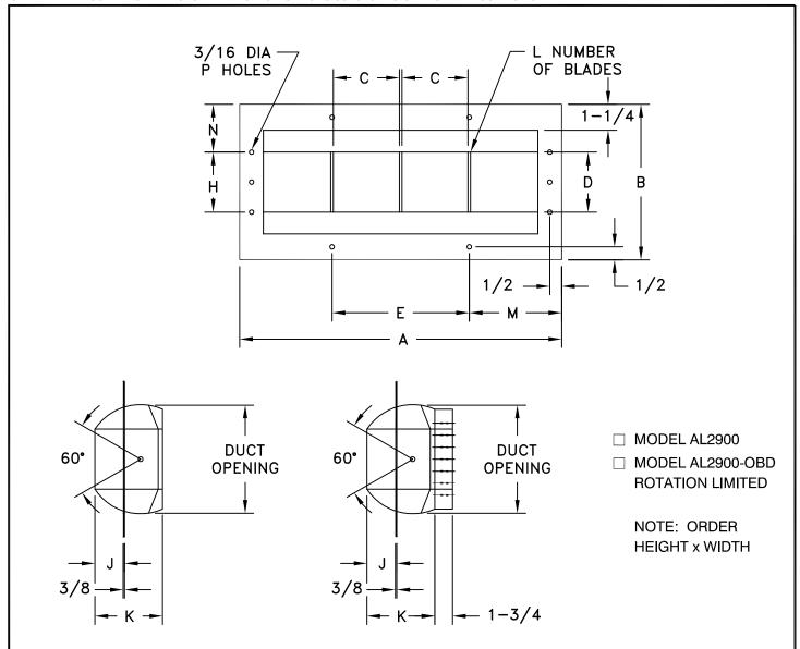
The Model AL2900 is ideal where extremely long throws are required with minimum ductwork. Adjustable drum and vane design provide horizontal or vertical air stream and throw control. The Model AL2900 is available with a screwdriver operated galvanized opposed blade damper to insure exacting volume control. Aluminum construction. Finish is white (W) or Mill (M).
