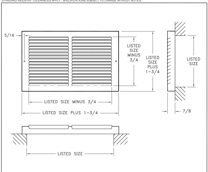
Model 60-GH-7 is a stamped face straight blade return for baseboard applications featuring one piece, steel construction with 7/8" turnback margins. Fins are spaced on 1/2" centers. Standard finish is white.
