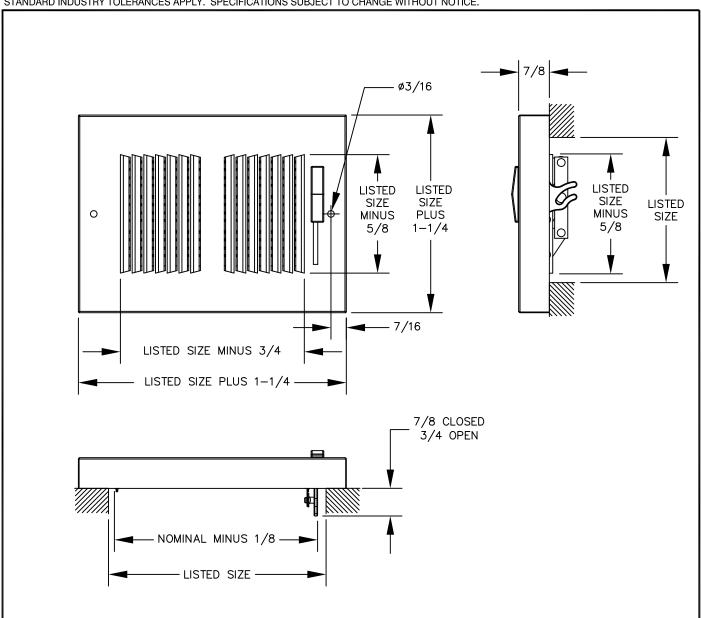
Model 667 is a stamped straight blade baseboard register with mounting holes. Constructed of steel with 1/3 inch fin spacing set at 45 degrees, it features a multi-louvered damper. Standard finish is white.
