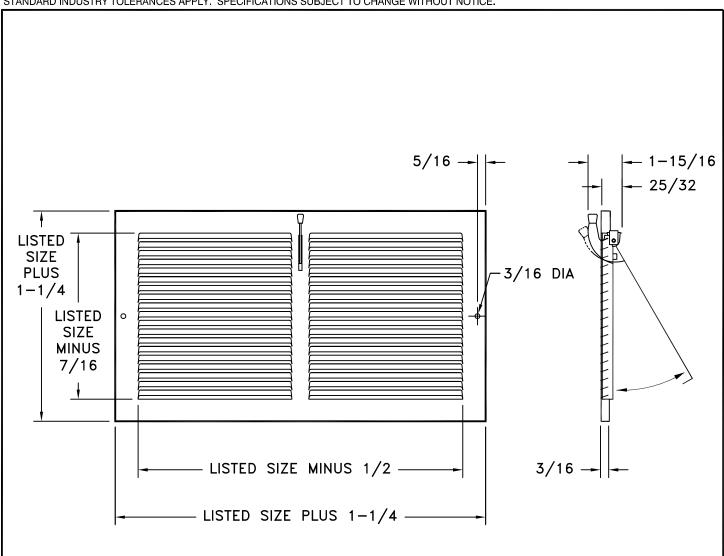
Model 653 is a stamped straight blade ceiling or sidewall register with mounting holes. Constructed of steel with 1/3 inch fin spacing set at 20 degrees, it features a plate style damper. Standard finish is white.
