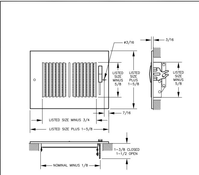
Model 632 is a two-way stamped straight blade ceiling or sidewall register with mounting holes. Constructed of steel with 1/3 inch fin spacing set at 45 degrees, it features a multi-louvered damper. Standard finish is white.
