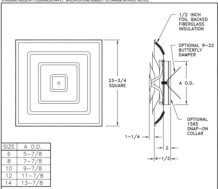
The Model 1560 is a high volume, 360 degree, 4-way fixed pattern ceiling diffuser that fits standard 2' x 2' T-Bar ceilings. For 6" - 12' flex duct applications, use corresponding 1565 collar. 14" size includes factory installed collar. Optional R-22, butterfly damper is available. Steel construction. Standard finish is white.
