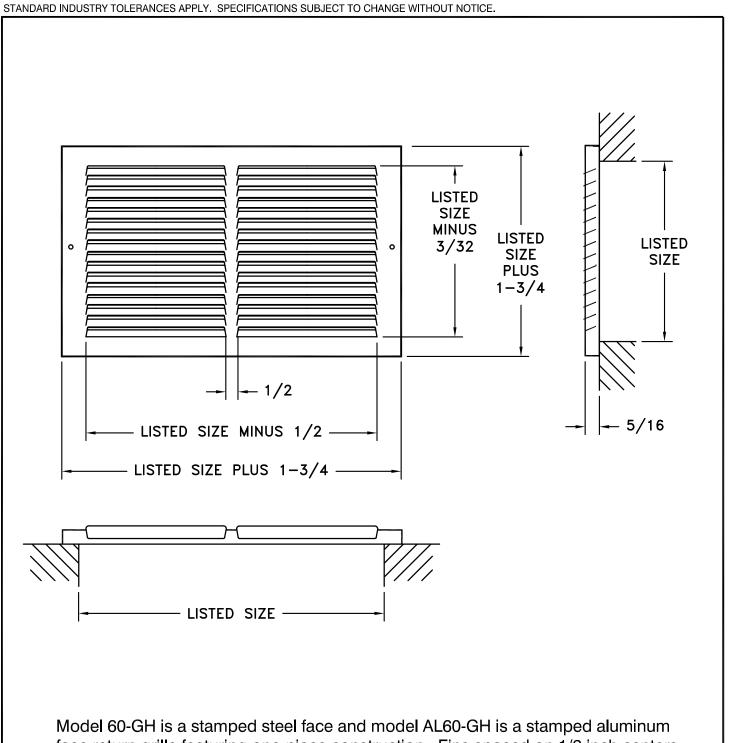
Model 60-GH is a stamped steel face and model AL60-GH is a stamped aluminum face return grille featuring one-piece construction. Fins spaced on 1/2 inch centers and set at 40 degrees. Standard finish is white for steel and mill for aluminum.
