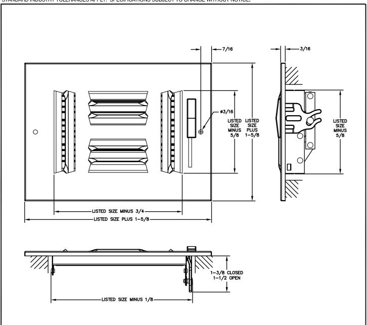
Model 604/AL604 is a stamped straight blade supply for ceiling installation. The Model 604/AL604 features a 4-way air deflection pattern. The steel multi-louvered damper assures equal air distribution over the diffuser face. Fins spaced at 1/2" and set at 45 degrees. Available in steel or aluminum. Standard finish is white.
