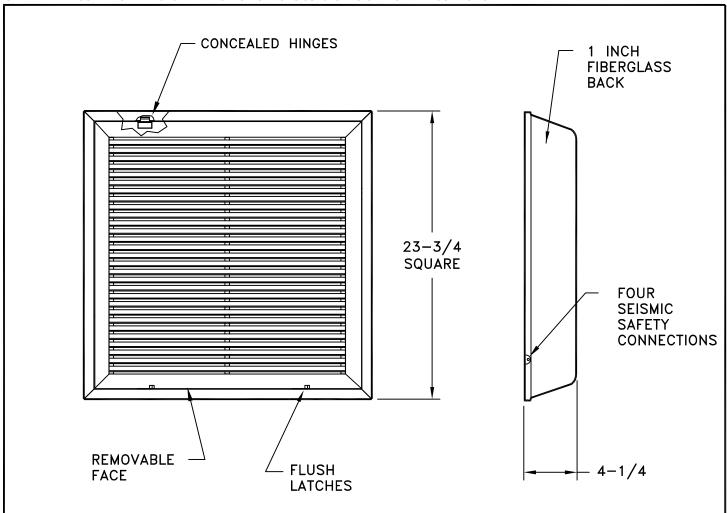
Model S90HFFI T-Bar Filter Grille is designed for use in all types of air conditioning systems. Standard fastening is flush latches located on side opposite hinge. Standard filter frames holds 1" disposable filter (provided by others). Steel construction. This model includes a molded fiberglass back with an R4.2 insulation value and integral adjustable filter retainers. Standard finish is white.
