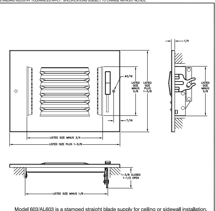
Model 603/AL603 is a stamped straight blade supply for ceiling or sidewall installation. The Model 603/AL603 features a 3-way air deflection pattern. The steel multi-louver damper assures equal air distribution over the diffuser face. Fins spaced at 1/2" and set at 45 degrees. Available in steel or aluminum. Standard finish is white.
