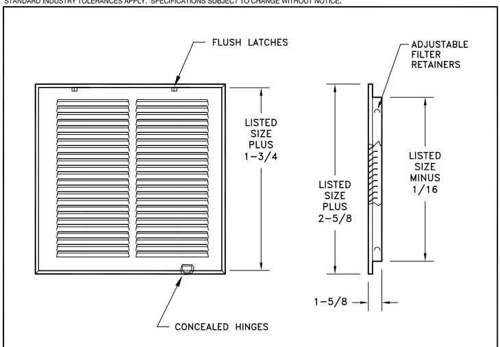
Model 60-GH-FF is a filter frame with a removable stamped face that is designed for use in air handling systems. In addition to holding the filter, it can be used as an access to the air handling unit. The filter frame holds standard 1" disposable filters (by others). T-Bar Frame optional. Steel construction only. Standard finish is white.
