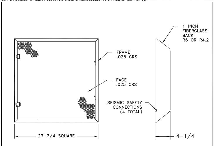
Model 12PFFI is a filter frame with a perforated face for use in all types of air conditioning systems with T-Bar ceilings. It acts as a holder for the filter or as an access opening into smaller air handling units. The filter frame holds standard one-inch disposable filters which are furnished by others. Steel construction. This model includes a molded fiberglass back with an R4.2 or R6 insulation value. Standard finish is white.
