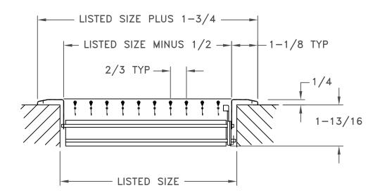
Model AL 278 aluminum register is available with individually adjustable straight blades for deflection control. The multi-louver damper allows additional volume control. The stamped face margins eliminate mitered corners and rough edges. Aluminum construction. Standard finish is white.
