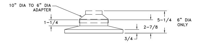
Model RZRNA is made from an Engineered ABS Polymer. Model RZRNA is a square to round adapter for the RZ1400. Model RZRNA is available in 6", 8", 10", 12" and 14" sizes. R22 and R42 dampers will fit RZRNA and must be field installed for a secure fit. Flexible Duct easily installs over round neck or RZRNA and is held in place with 3 retaining clips on top edge of neck.
