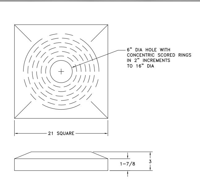
Model RZPL is made from an Engineered ABS Polymer. Model RZPL is a back panel for the RZ1444. Model RZPL can adapt to fit 6", 8", 10", 12", 14" and 16" collars. Installer cuts pre-scored rings to adapt the back panel to 8" through 16". Standard finish is white.
