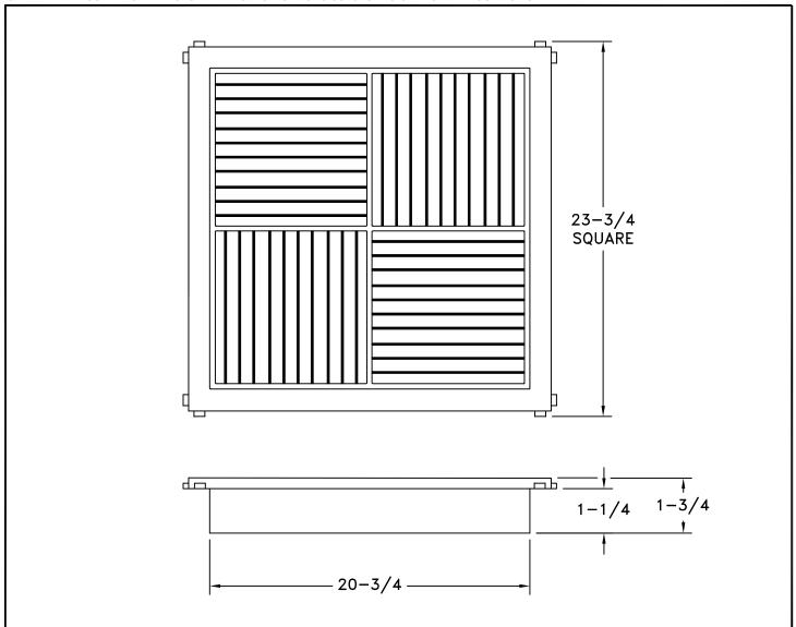
Model RZ1444 is made from an Engineered ABS Polymer. Model RZ1444 is a square modular supply or return diffuser. The unit's modular cores provide 1, 2, 3, 4 or 2-way corner pattern deflection. Removable modules provide easy access to accessories. Model RZ1444 will accept the Model RZPL back panel (ordered separately). Standard finish is white.
