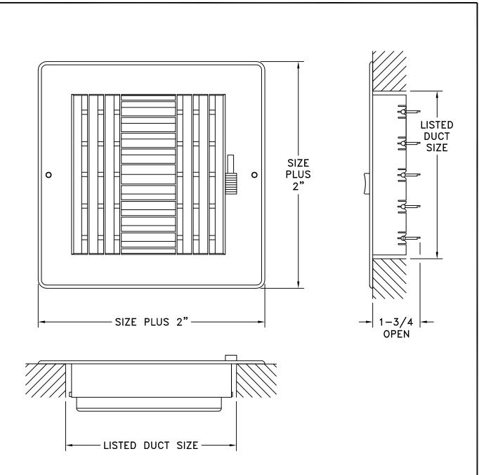
Model RZ604 is made from an Engineered ABS Polymer. Model RZ604 is a 4-Way straight blade supply for ceiling or sidewall installation and includes a multi-louver damper for volume control. Ideal for heating or cooling. Standard finish is white.
