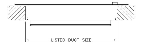
Model RZ602 is made from an UV Engineered ABS Polymer. Model RZ602 is a 2-way straight blade supply for ceiling or sidewall installation and includes a multi-louver damper for volume control. Ideal for heating or cooling. Standard finish is white.
