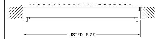
Model RZ800 is a solid ABS construction for floor use. RZ800 has multi-angled fins for a fan pattern of air distribution, and a foot operated multi-louver damper for volume control. Available in white or brown finish.
