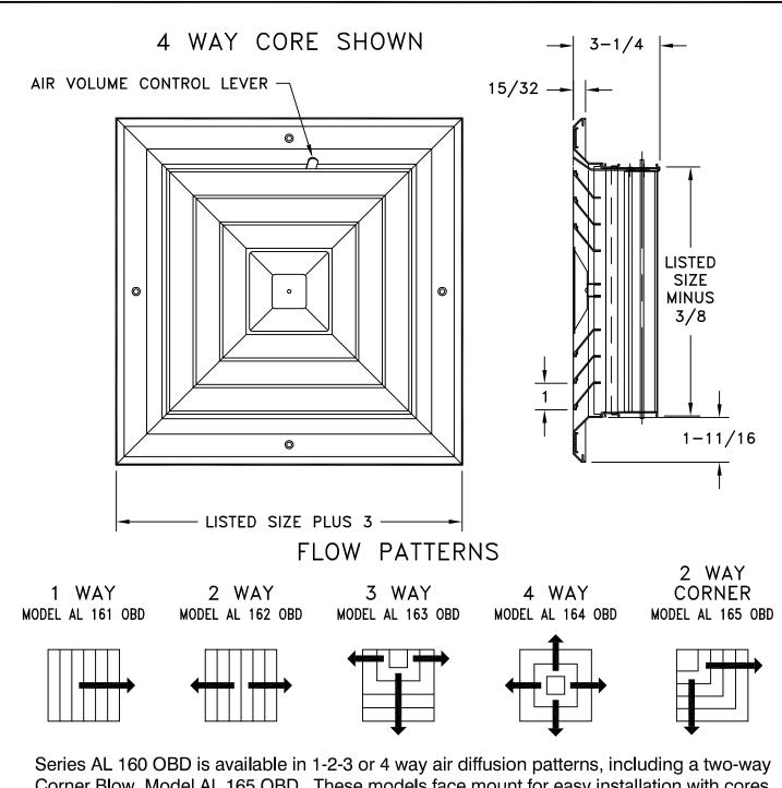
Series AL 160 OBD is available in 1-2-3 or 4 way air diffusion patterns, including a two-way Corner Blow, Model AL 165 OBD. These models face mount for easy installation with cores flush with margin. Series AL 160 OBD is designed for ceiling installations and includes an opposed blade damper. Extruded aluminum construction. Standard finish is white.
