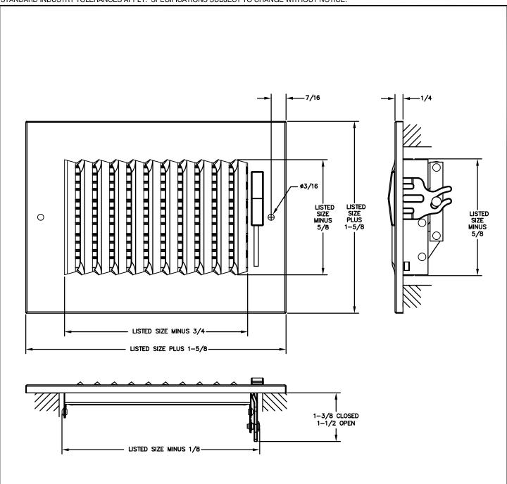
Model 602/AL602 is a stamped straight blade supply for ceiling or sidewall installation. The 602/AL602 features a one-piece faceplate with a multi-louver steel damper for volume control. Fins spaced at 1/2" and set at 45 degrees. Two way deflection is ideal for heating or cooling. Available in steel or aluminum. Standard finish is white.
