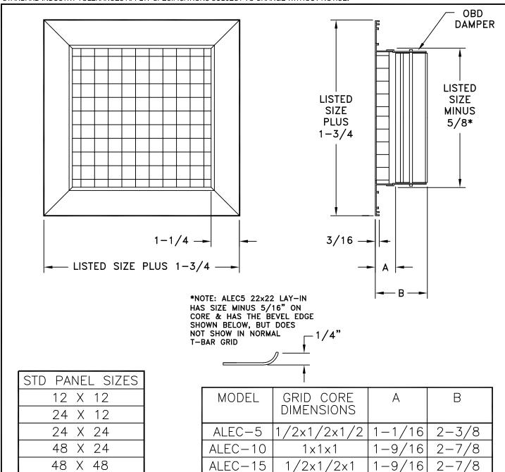
The Models ALEC-5, -10, -15 with frame 33 are T-bar return air grilles that have an aluminum square pattern grid providing maximum free area and minimum see through. The optional opposed blade damper (OBD) is offered in steel with aluminum as another option. Standard finish is white.
