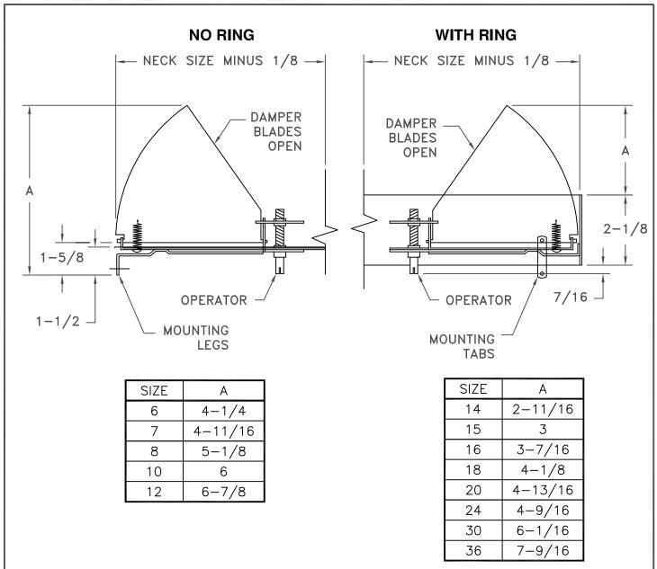
Model R-32 dampers feature gang operated radial blades that move in right angles to the air flow to regulate air volume. A flat configuration with no adapter ring enables the damper to be mounted flush with the neck of diffuser. Adjustments are easily made from the face of the diffuser with a screwdriver. Available in 6" thru 36". Steel construction. Mil Finish.
