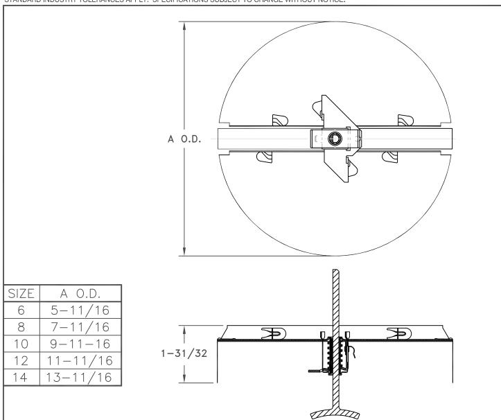
Model R-22 Round butterfly damper is designed to be use with most round neck diffusers for efficient volume control. The R-22 can be adjusted from the face of the diffuser with a nylon T handle that is provided. The damper is designed for quick and easy attachment to the neck and is shipped separate from the diffuser. Available in 6", 8", 10", 12" and 14". Steel construction. Brown Finish.
