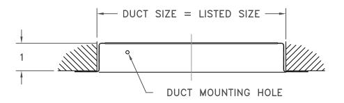
Model 156 Duct Ring only. Steel construction. Standard finish is brown. For use with Model 150.
