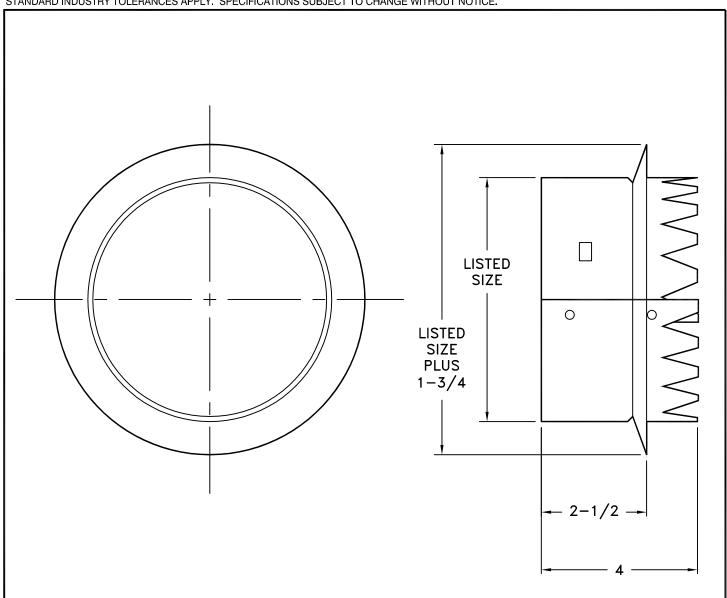
The Model R12 Spin-In Collar is designed for use on molded fiberglass and duct board backs. This galvanized collar accepts R22, R32 and R42 round neck dampers. Available sizes are 6, 8, 10, 12 and 14-inch diameters.
