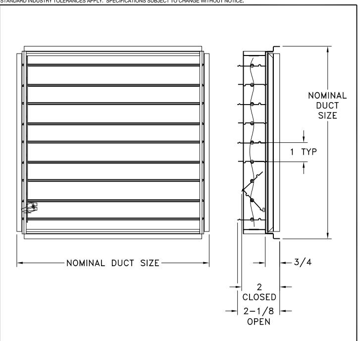
Model OBD-14 is used to control air flow at the diffuser. Duct mount ONLY if ordered separately. Available in 3 inch increments from 6 x 6 to 24 x 24. Must remove core with flat screwdriver. Steel construction. Standard finish is white.
