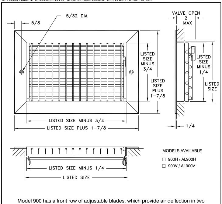
directions. Blades are spaced at 3/4" and are spring stiffened at both ends to permit positive setting without special tools. Lever operated multi-louver damper blades interlock when closed. Steel construction. Standard finish is white.
