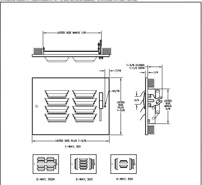
The Series 500/AL500 is a stamped curved-blade supply register for ceiling or sidewall installation featuring a multi-louver damper for volume control. It is available in four air flow patterns and offers steel or aluminum face construction. Standard finish is white.
