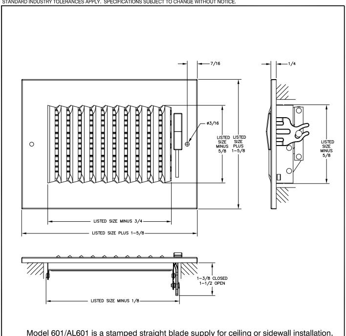
Model 601/AL601 is a stamped straight blade supply for ceiling or sidewall installation. The 601/AL601 features a one-piece faceplate with a steel multi-louver damper for volune control. Fins spaced at 1/2" and set at 45 degrees. One way deflection is ideal for heating and cooling. Available in steel or aluminum. Standard finish is white.
