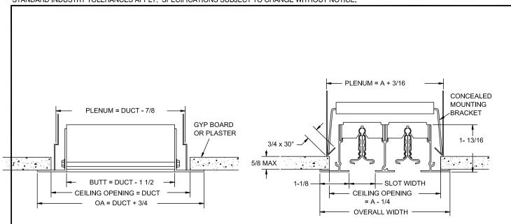
• CONTRACTOR TO FRAME OPENING TO INSURE STRAIGHT LINE INSTALLATION (TYPICAL ALL INSTALLATIONS)
