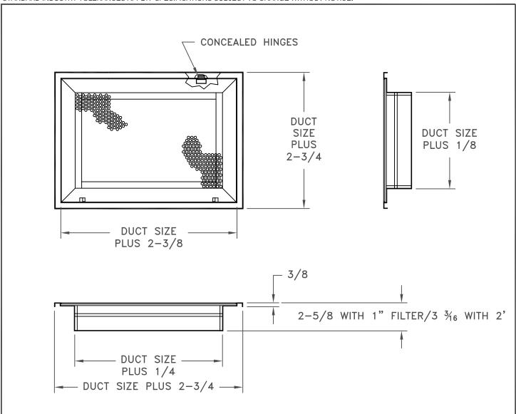
Model 12P-FF is a filter frame with a perforated face for use in all types of air conditioning systems. It acts as a holder for the filter or as an access opening into smaller air handling units. The perforated grille face is hinged parallel to the horizontal dimension unless otherwise specified. The filter frame holds standard one-inch disposable filters which are furnished by others. Steel construction. Standard finish is white.
