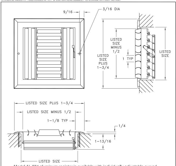
Model AL 274 aluminum register is available with individually adjustable curved blades for increased deflection control. Model AL 274 four-way deflection is designed for sidewall or ceiling application. The stamped face of Model AL 274 eliminates mitered corners and potential rough edges. Multi-louver damper assembly included. Aluminum construction. Standard finish is white.
