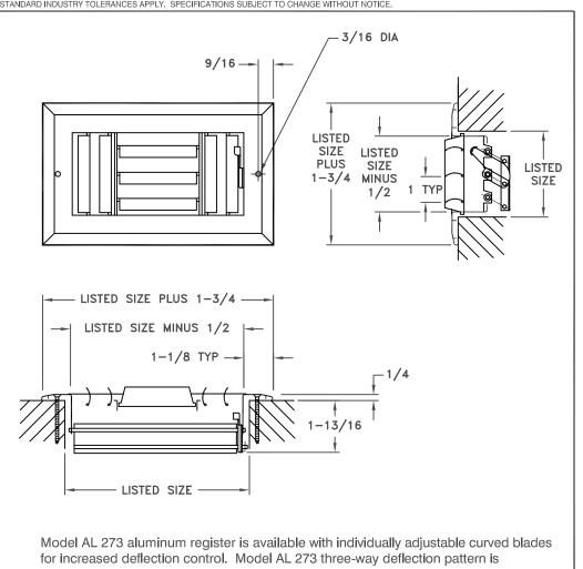
designed for sidewall or ceiling application. The stamped face of Model AL 273 eliminates mitered corners and potential rough edges. Multi-louver damper assembly included. Aluminum construction. Standard finish is white.
