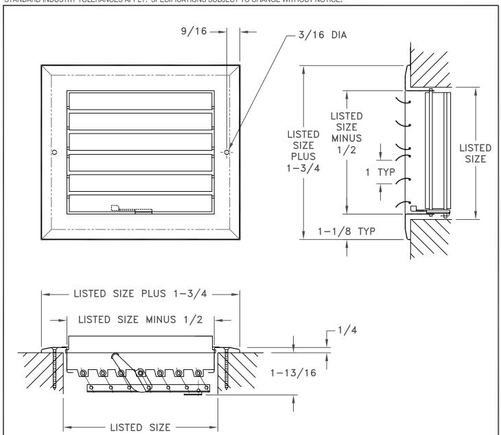
Model AL 272 aluminum register is available with individually adjustable curved blades for increased deflection control. The two-way deflection pattern is designed for sidewall or ceiling application. The stamped face of Model AL 272 eliminates mitered corners and potential rough edges. Multi-louver damper assembly included. Aluminum construction. Standard finish is white.
