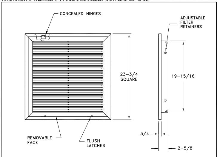
Series S90HFF Grille with T-Bar filter frame is designed for use in T-Bar Ceilings. Grille face hinged on top for easy access to filter. Standard fastening is flush latches located on side opposite hinge. Standard filter frames holds 1" disposable filter (provided by others). 2" and 4" filter sizes also available. Steel construction. Standard finish is white.
