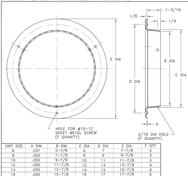
Pre-drilled mounting holes allows duct ring to be easily attached to duct.
