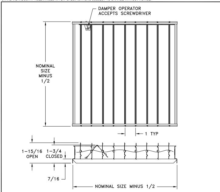
Model OBD is constructed of galvanized steel with vertical blades that simultaneously move in opposite directions to provide uniform air distribution over the entire diffuser face. Tension spring interwoven on blade pivot points permits positive damper setting in any position from fully open to fully closed. Damper blades are screwdriver operated. Extremely shallow depth allows damper to be used in shallow stackheads. Steel construction. Mill finish.
