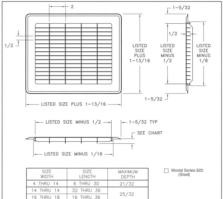
The Model 825 is a bar return with heavy gauge interlocking bars on 1/2" and 2" centers. Steel construction only. Standard finish is brown.
