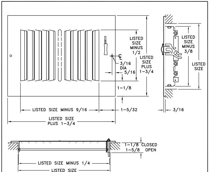
Model 602/AL602 is a stamped straight blade supply for ceiling or sidewall installation. The 602/AL602 features a one-piece faceplate with a multi-louver steel damper for volume control. Fins spaced at 1/2" and set at 40 degrees. Two way deflection is ideal for heating or cooling. Available in steel or aluminum. Standard finish is white.
