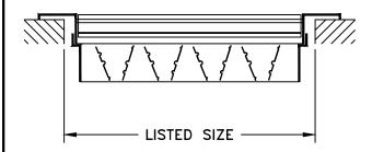
Model ALS90Z is a matching return air unit for Series 90, 990 and 900 supply units. Optional Opposed Blade Damper (OBD) ensures exacting volume control by spreading air uniformly. Damper is screwdriver operated. Aluminum construction with steel OBD (standard aluminum AL-OBD optional). Standard finish is white.
